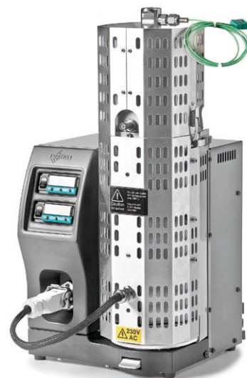
Heating unit of the High Temperature ELPI®+
