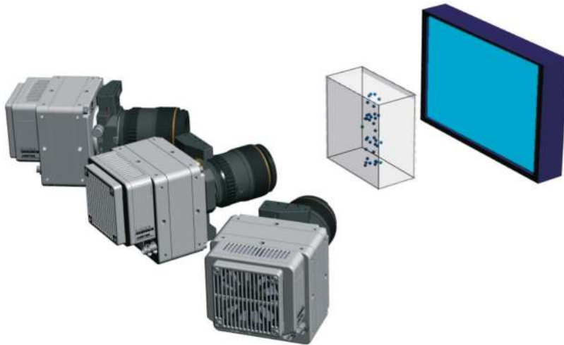
High-speed tomographic shadow imaging in multiphase flows
