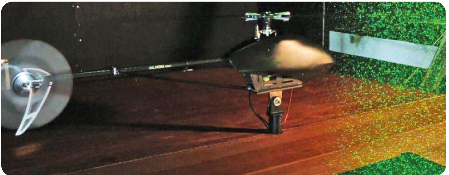
Shake-the-Box experiment: helicopter in ground effect (courtesy DLR)
